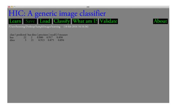
The formatting is not perfect, but readable. We notice, e.g., that out of 24 true busses, 22 of them are classified correctly and 2 wrongly. For bus recognition, the recall of this trained model is 0.880, the precision 0.917 and the f measure 0.898.
